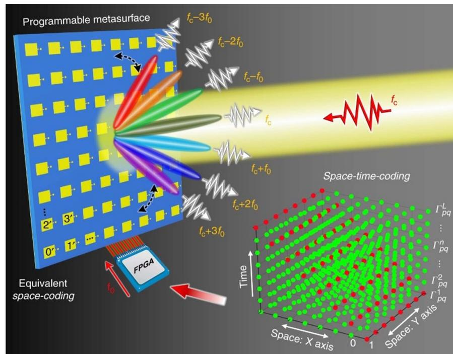
**Figure 65.** Conceptual illustration of a space-time-coding digital metasurface that can simultaneously manipulate EM waves in both space and frequency domains, i.e. control the propagation direction and harmonic power distribution simultaneously. Reproduced from [11]. CC BY 4.0.
