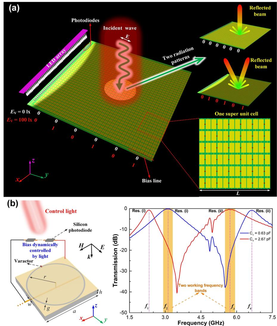
**Figure 61.** Two photodiode-based light-controlled programmable metasurfaces that are used for controlling (a) the reflection beams and (b) the transmission amplitude of EM waves in a real time. Reproduced from [415]. CC BY 4.0. Reprinted from [416], with the permission of AIP Publishing.
