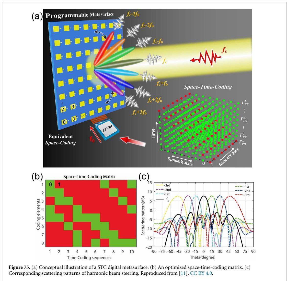
**Figure 75.** (a) Conceptual illustration of a STC digital metasurface. (b) An optimized space-time-coding matrix. (c) Corresponding scattering patterns of harmonic beam steering. Reproduced from [11]. CC BY 4.0.
