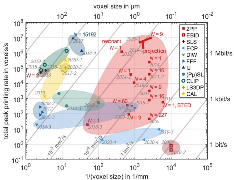
**Figure 10.** Comparison of 3D additive manufacturing approaches suitable for making 3D metamaterials in terms of 3D printing rate and voxel size. [61] John Wiley & Sons. © 2020 The Authors. Published by WILEY-VCH Verlag GmbH & Co. KGaA, Weinheim.
