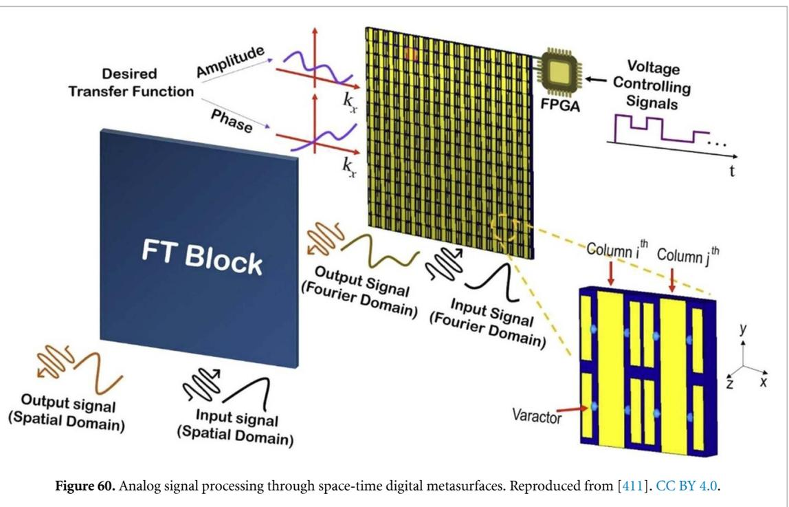
**Figure 60.** Analog signal processing through space-time digital metasurfaces. Reproduced from [411]. CC BY 4.0.
