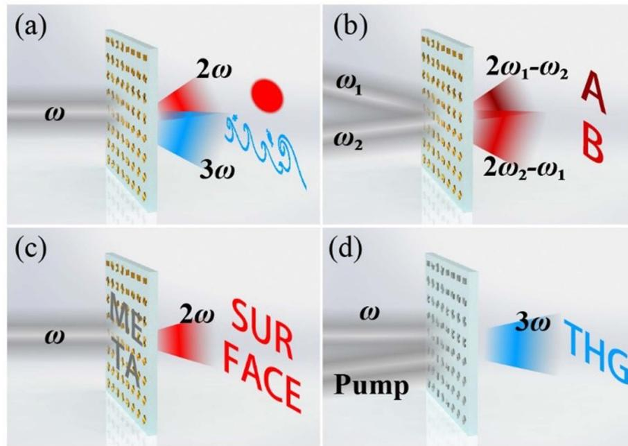
**Figure 35.** Advances of nonlinear metasurface holography. (a) Bi-color nonlinear metasurface holography. (b) Four wave mixing holographic multiplexing. (c) Nonlinear metasurface for real and Fourier space imaging encoding. (d) Expectation of switchable nonlinear metasurface holography.
