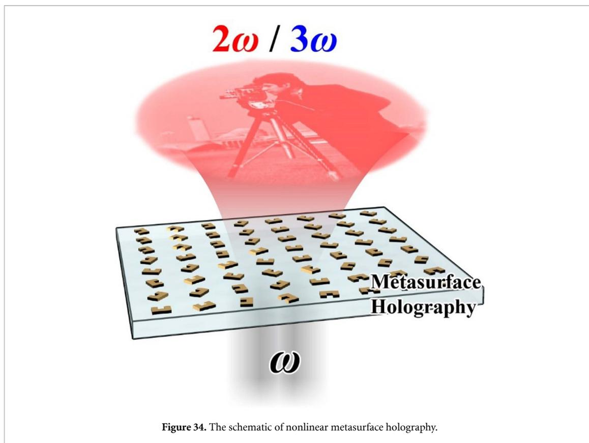
Figure 34. The schematic of nonlinear metasurface holography.
