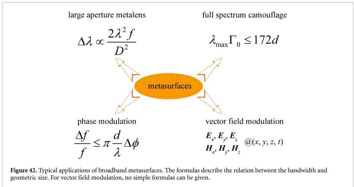
Figure 42. Typical applications of broadband metasurfaces. The formulas describe the relation between the bandwidth and geometric size. For vector field modulation, no simple formulas can be given.
