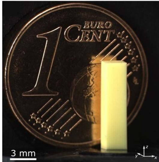
**Figure 9.** Photograph of a 3D chiral elastic metamaterial containing more than 105 3D unit cells and more than  $3 \times 10^9$  voxels. A Euro cent coin serves for reference. [61] John Wiley & Sons. © 2020 The Authors. Published by WILEY-VCH Verlag GmbH & Co. KGaA, Weinheim.
