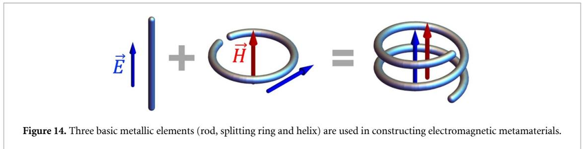
Figure 14. Three basic metallic elements (rod, splitting ring and helix) are used in constructing electromagnetic metamaterials.
