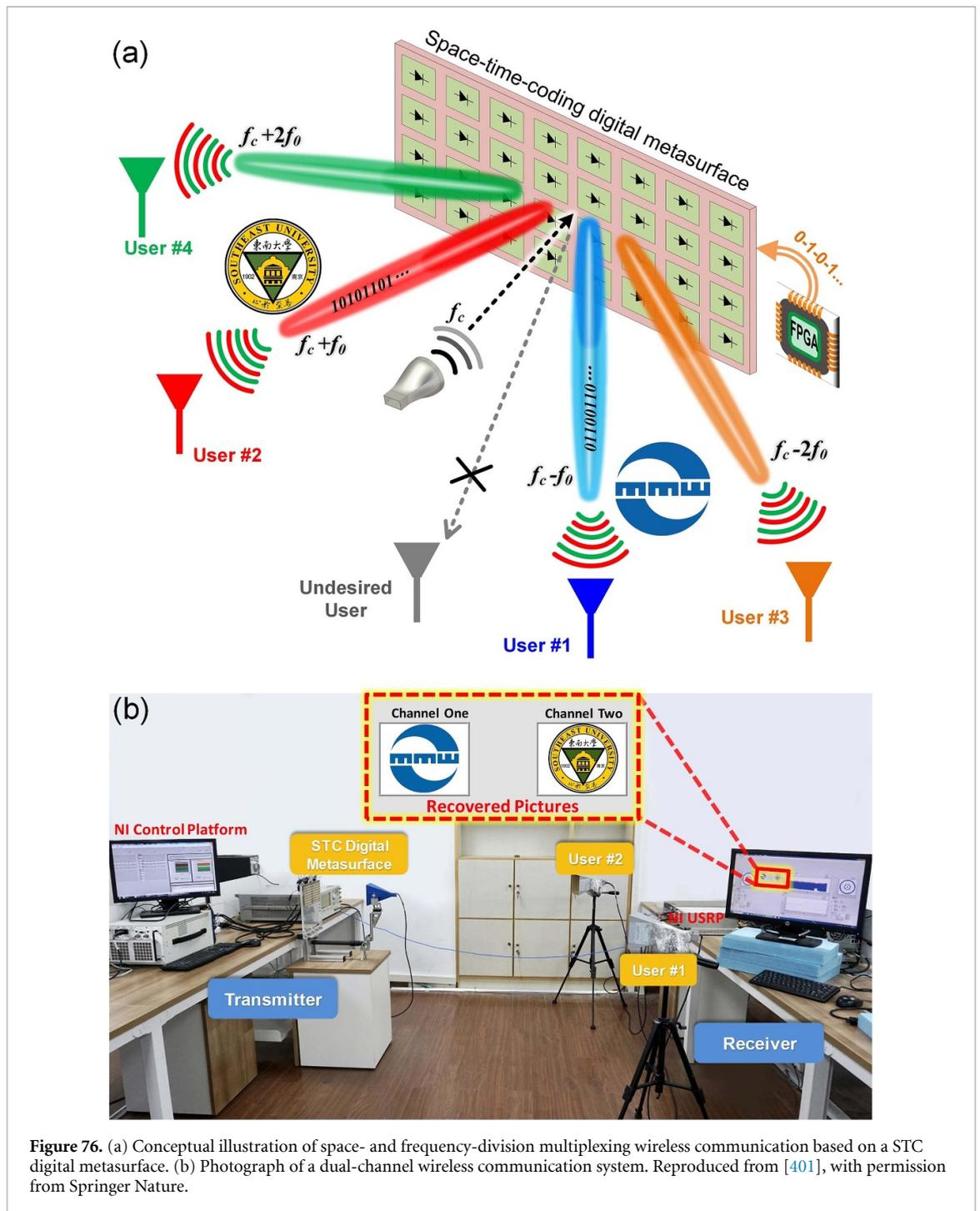
**Figure 76.** (a) Conceptual illustration of space- and frequency-division multiplexing wireless communication based on a STC digital metasurface. (b) Photograph of a dual-channel wireless communication system. Reproduced from [401], with permission from Springer Nature.
