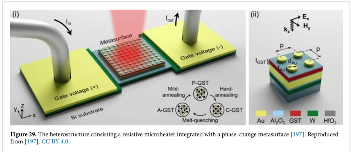
**Figure 29.** The heterostructure consisting a resistive microheater integrated with a phase-change metasurface [197]. Reproduced from [197]. CC BY 4.0.
