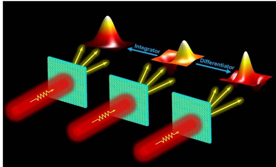
**Figure 59.** Mathematical operations of transmissive near fields controlled by metasurface with phase and amplitude modulations. [410] John Wiley & Sons. © 2020 WILEY-VCH Verlag GmbH & Co. KGaA, Weinheim.
