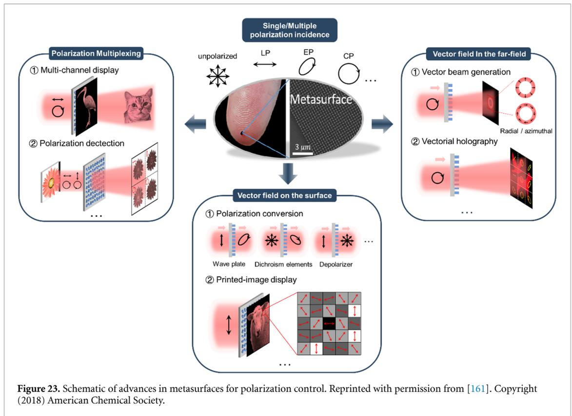
**Figure 23.** Schematic of advances in metasurfaces for polarization control. Reprinted with permission from [161]. Copyright (2018) American Chemical Society.
