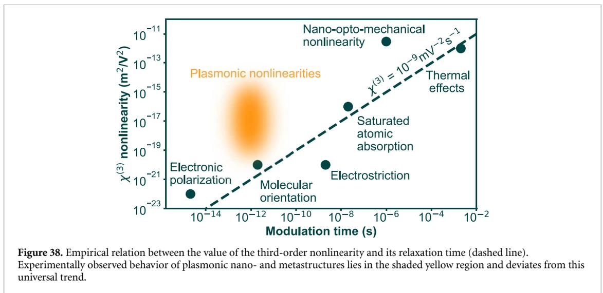
Figure 38. Empirical relation between the value of the third-order nonlinearity and its relaxation time (dashed line). Experimentally observed behavior of plasmonic nano- and metastructures lies in the shaded yellow region and deviates from this universal trend.
