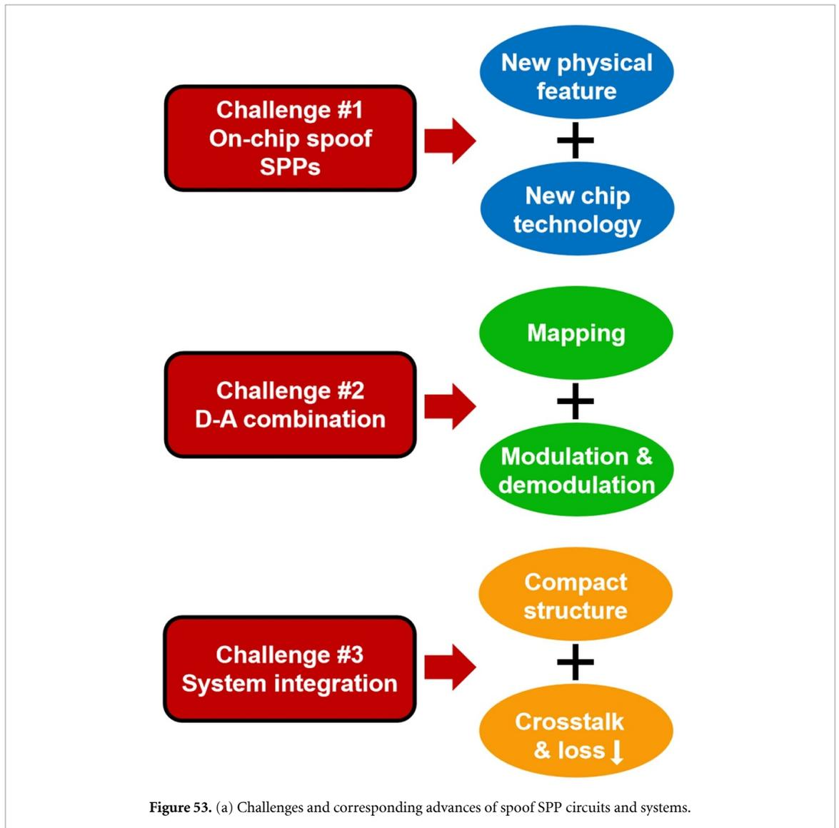
Figure 53. (a) Challenges and corresponding advances of spoof SPP circuits and systems.
