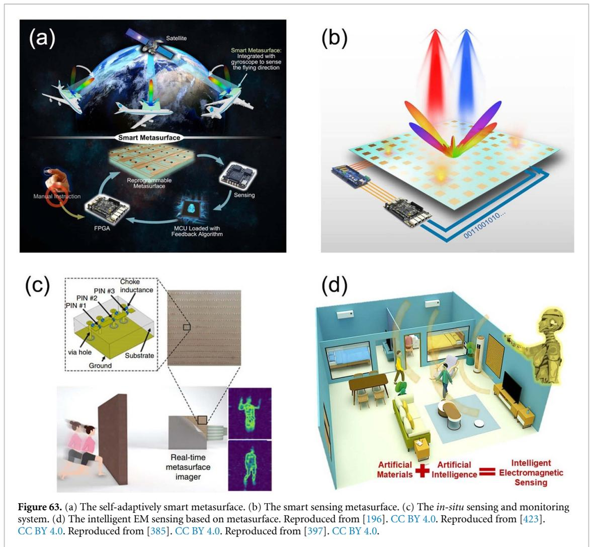
**Figure 63.** (a) The self-adaptively smart metasurface. (b) The smart sensing metasurface. (c) The *in-situ* sensing and monitoring system. (d) The intelligent EM sensing based on metasurface. Reproduced from [196]. CC BY 4.0. Reproduced from [423]. CC BY 4.0. Reproduced from [385]. CC BY 4.0. Reproduced from [397]. CC BY 4.0.
