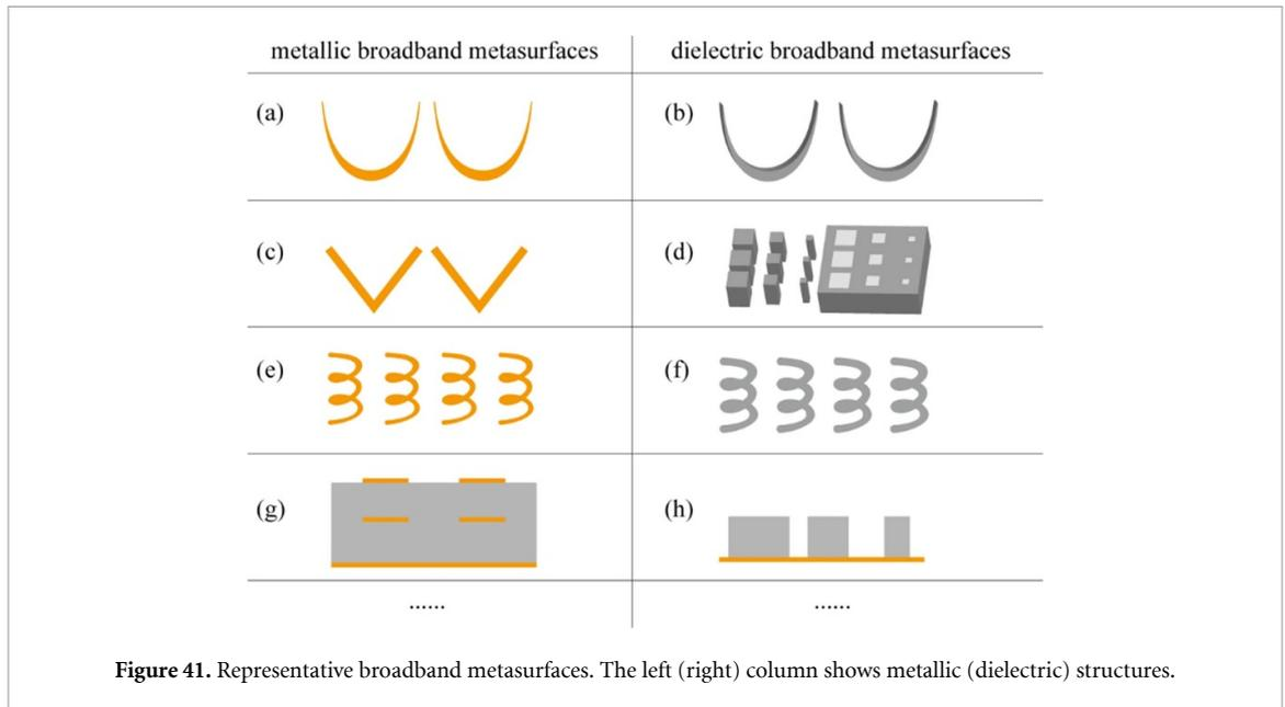
Figure 41. Representative broadband metasurfaces. The left (right) column shows metallic (dielectric) structures.
