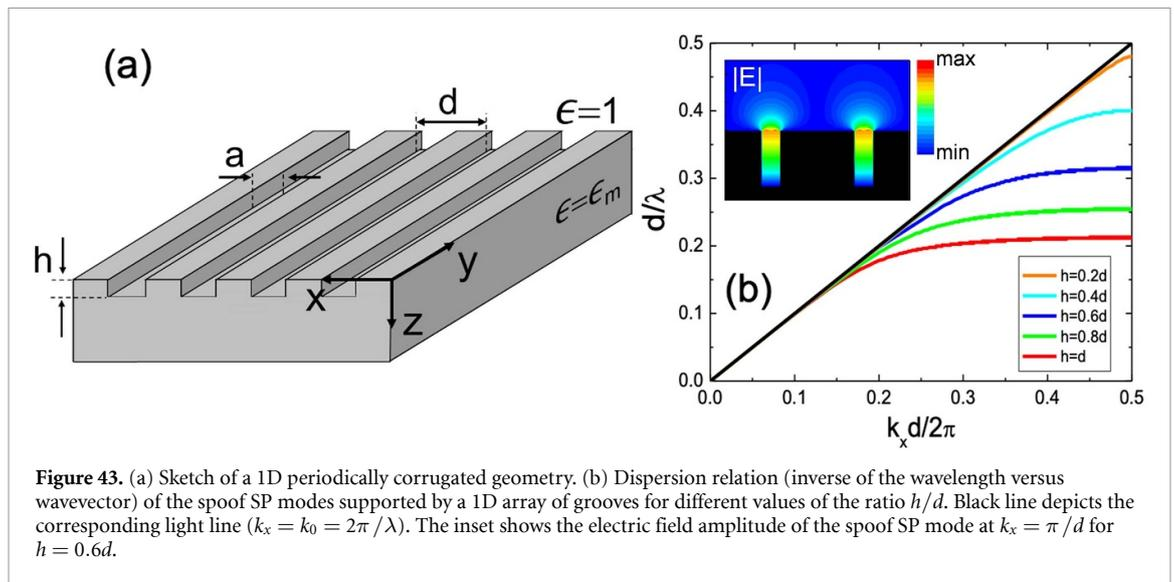
**Figure 43.** (a) Sketch of a 1D periodically corrugated geometry. (b) Dispersion relation (inverse of the wavelength versus wavevector) of the spoof SP modes supported by a 1D array of grooves for different values of the ratio  $h/d$ . Black line depicts the corresponding light line ( $k_x = k_0 = 2\pi/\lambda$ ). The inset shows the electric field amplitude of the spoof SP mode at  $k_x = \pi/d$  for  $h = 0.6d$ .
